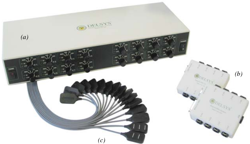
Figure 4: (a) The Bagnoli-16 Main Amplifier Unit. (b) Input Modules. (c) DE Series electrodes.
